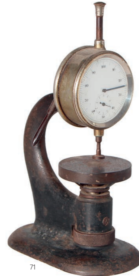
70 Twist Meter Manufacturer / Model: Stagionatura Anonima Year: Before 1926 Dimensions: 17 × 130 × 20 cm Inventory No.: 2024/3/4 (1994/1/33-1)
