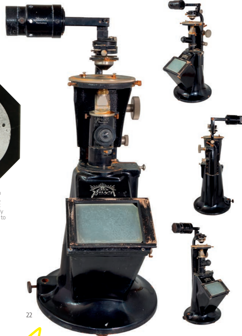
The Busch Metaphot 400, slightly larger than any microscope of its time, represented a major breakthrough in the field of macro- and microphotography, as it greatly reduced the space previously required by the bulky optical benches (which could reach several metres in length). The Metaphot was compatible with objectives and eyepieces from different manufacturers and could be fitted with additional accessories such as colour filters, focusing magnifiers, and various drawing devices.
