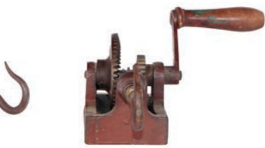
72 Hand-crank Strand Twister Manufacturer / Model: Unknown Year: Early 20th century Dimensions: 16 × 38 × 24 cm Inventory No.: 2024/3/13-2
