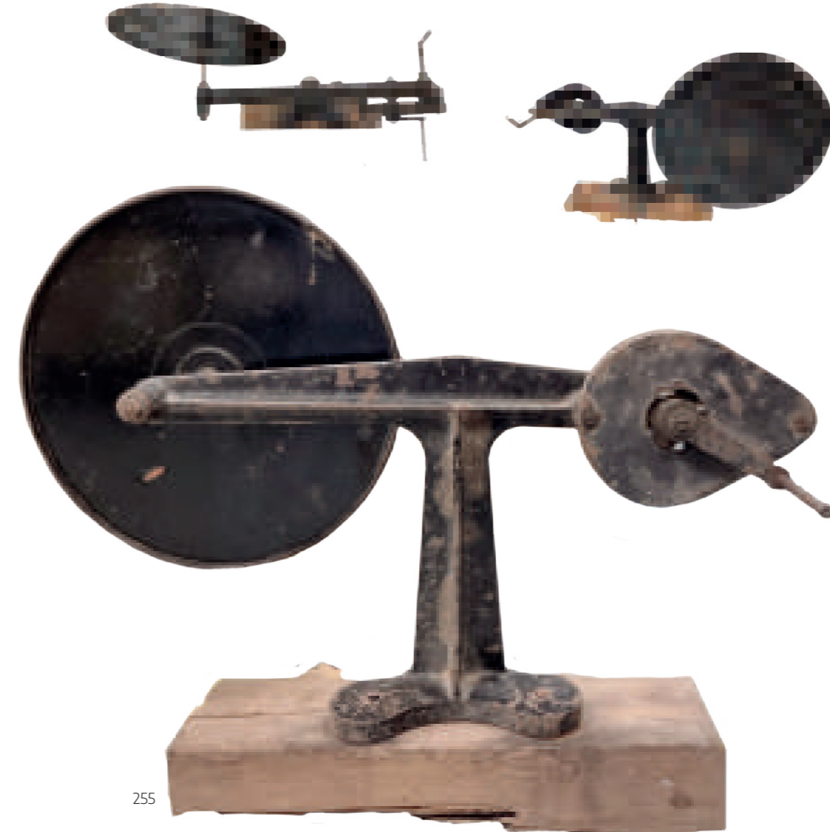
255 35 mm Film Rewinder Brand/Model: Pathé Machine Ref. 9/300 Year: 1919 Dimensions: 41 x 56 x 27 cm Inventory No.: 2024/8/15
