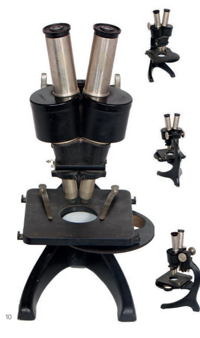
10 Stereoscopic Microscope Manufacturer / Model: Carl Zeiss Greenough Serial No.: 203882 Year: 1912 Dimensions: 32 × 14 × 19 cm Inventory No.: 2024/2/5-6 (1994/1/33/6)
