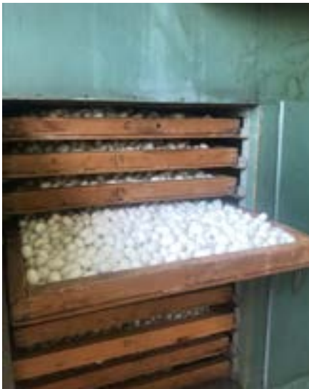
CREA – Sericulture Lab – Electric cocoon dryer (Source / CREA Sericulture laboratory , Padua)
