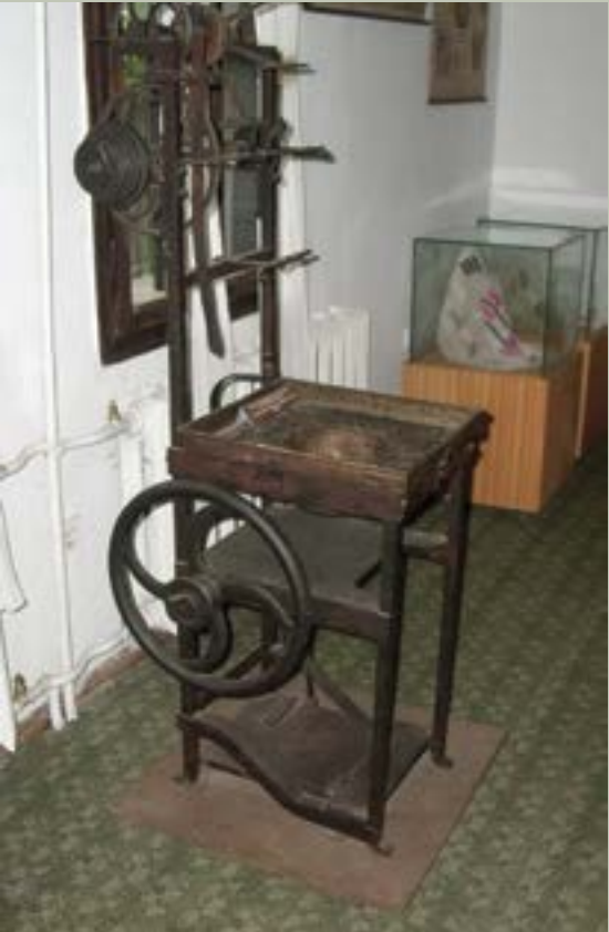
Right: Manual silk reeling tool, used at the end of the 19th century (Source: Vratsa's Ethnographic Museum). Left: Improved Vratsa's type manual silk reeling tool, beginning of the 20th century (Source / Vratsa's Ethnographic Museum)
