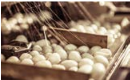
Reeling of cocoons after cooking, brushing, end picking (Source / D’orica, Nove (VI), Italy)
