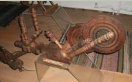
Right and left: Home manual wheel for silk twisting, first half of the 20th century (Source: SES-Vratsa Sericulture exhibition )
