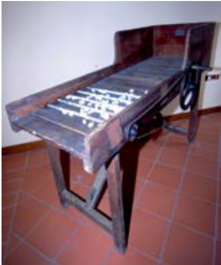
Traditional manual deflossing machine used to remove the floss or the outer silk cocoon layer (Source / Sericulture laboratory of CREA – Padua)
